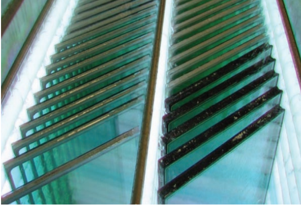
P-1 Test Chamber: 140°F, constant UV, water spray
